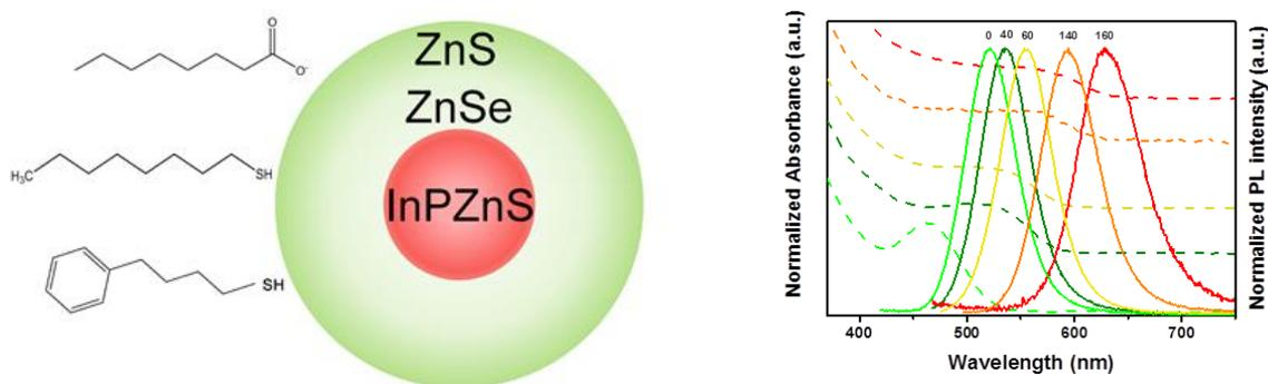
**Figure 1.** The structure of InPZnS/ZnSe/ZnS alloyed core/multishell quantum dots (left). The optical properties of InPZnS core with different peak wavelengths (right)
