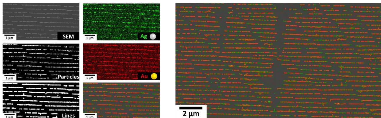
**Figure 1.** SEM-EDX and subsequent image analysis of the generated particle lines. Algorithms applied to the SEM image allow assigning each single particle to its corresponding line. A comparison of the silver and gold intensities integrated over each particle allows assigning particle composition, which can then be statistically analyzed.
