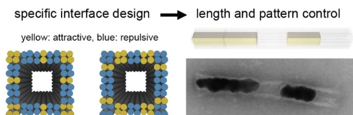
**Figure 1.** Sketch and tSEM images showing the modular DNA platform. With specific interface design by choosing different helix positions for attractive and repulsive reaction, the length and pattern of the metal structures can be controlled.
