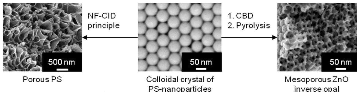
**Figure 1.** (Middle) SEM image of colloidal crystal of PS-nanoparticles used to (left) synthesize nanoporous PS following the NF-CID principle or (right) ZnO inverse opals via the CBD method. a
