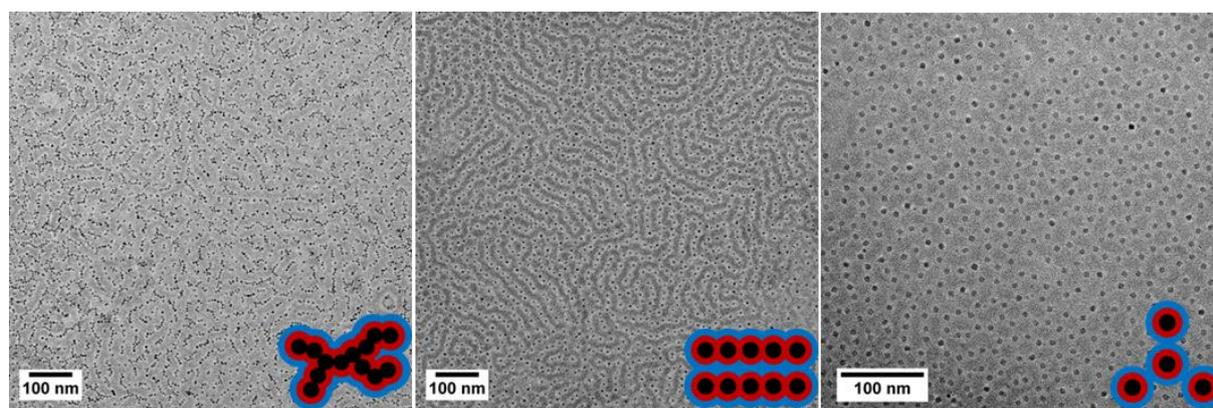
**Figure 1.** TEM images of different types of nanoparticle arrays which can be realized by variation of the grafting density of the block copolymers.
