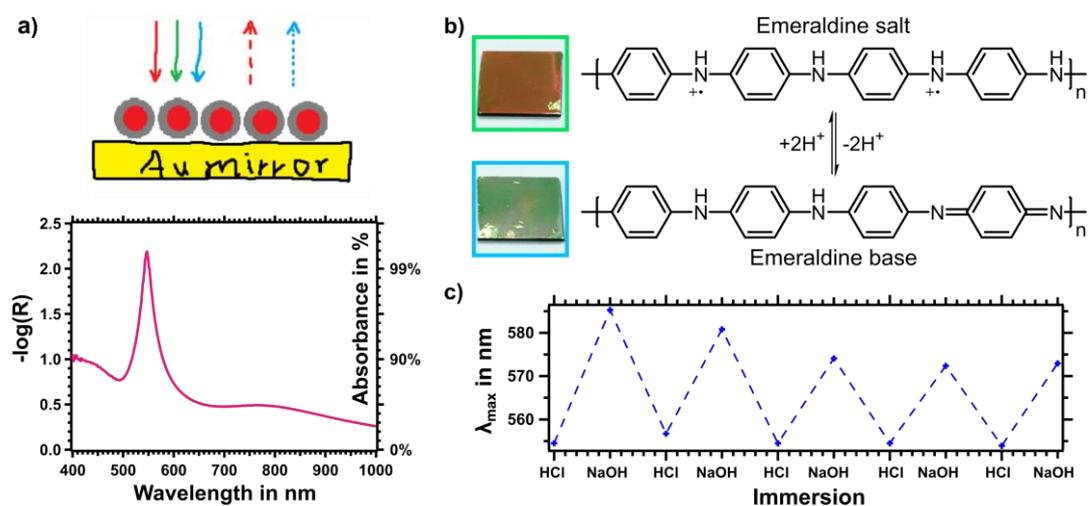
**Figure 1.** a) Scheme of the metasurface near-perfect absorber and its absorbance spectrum calculated from reflectance measurements at 10° incidence. b) Structural formula of the protonated form (emeraldine salt) and deprotonated form (emeraldine base) of polyaniline with respective photographs of the plasmonic metasurface. c) Maximum peak positions of the absorbance spectra after immersion in HCl or NaOH.
