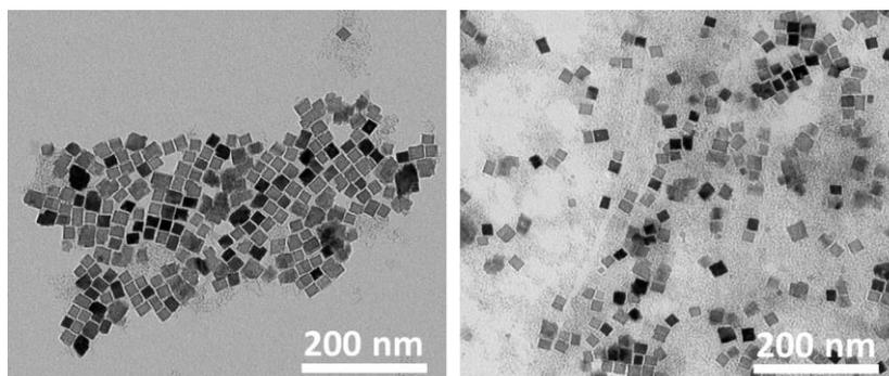
**Figure 1.** Representative TEM images of the BaTiO<sub>3</sub> cubic particles dispersed in toluene with oleic acid as surfactant.
