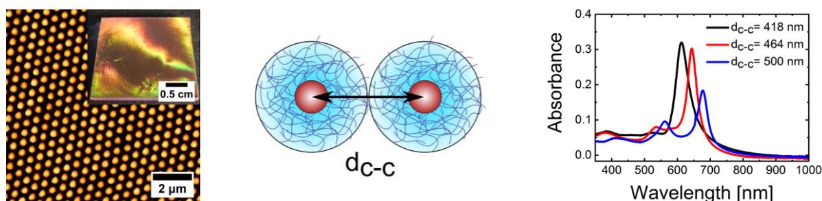
**Figure 1.** Left: Atomic force microscopy image of a representative ordered gold array. The inset shows a digital photograph of gold monolayer on a glass substrate. Middle: schematic view of core-shell particles with their nearest neighbor center-to-center distance  $d_{c-c}$ . Right: SLRs resonances of coated monolayers with varying  $d_{c-c}$ .
