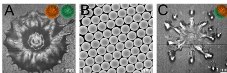
**Figure 1.** A) Representative optical image of the impact of a supercooled water droplet on a surface based on a mixture of two different particle types, B) SEM image of a particle-based surface, C) representative optical image of the impact of a supercooled water drop on a surface based on Janus particles.
