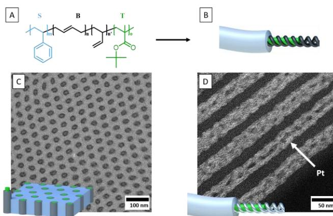
**Figure 1.** From core-shell cylinder morphology to double helices. A) Chemical structure of SBT. B) Schematic of cross-linked and unloaded helix-on-cylinder. C) SBT bulk film. D) Platinum loaded double helices.
