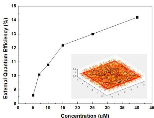
Figure 1. The simulated external quantum efficiency of LSCs under excitation (516nm) as a function of concentration of Lumogen Red 305. 10,000 photons were traced in each simulation. The insert illustrates one Monte-Carlo ray simulation of LSC at G=5.
