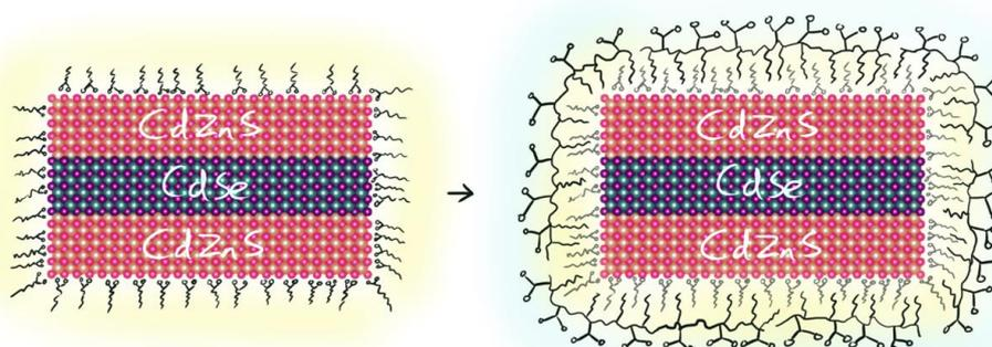
**Figure 1.** Illustration of polymer coating. Hydrophobic regions are highlighted in yellow.
