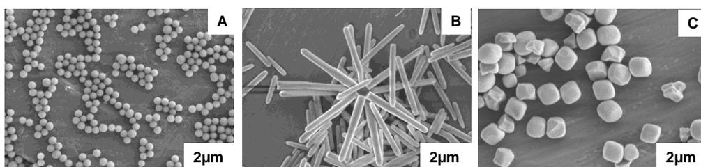
**Figure 1:** Scanning Electron Microscopy images of a) spherical, b) rod and c) cubic particles.
