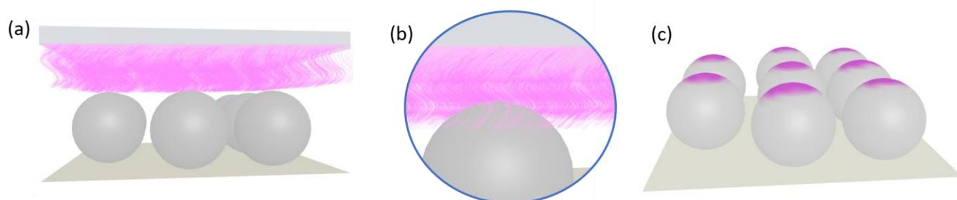
**Figure 1.** Schematic overview over the described microcontact printing process: (a) An inked, polymer brush-modified stamp approaches the particle monolayer; (b) Direct contact between particle surface and stamp facilitates the ink transfer mediated by the presence of the polymer; (c) Release of the patchy particles upon the removal of the stamp.
